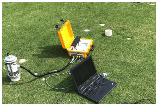
(Fig. 5) Carbon efflux measurements recorded with a LI-COR 8100A automated system.
