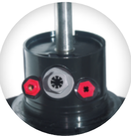
RISER REMOVAL TOOLS 995-85 Drive assembly extraction tool 730, 760, 780, 860S, 880S Threads onto the drive output shaft and allows removal of the drive from the body
