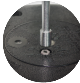
995-81 9/16" 760/780 Series Main 995-80 1/2" 760/780/860S/880S Nozzle base jam nut removal
