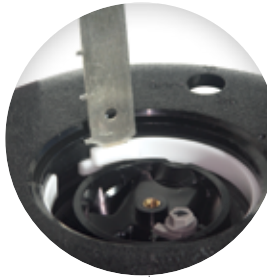
995-82 Upper snap ring remover on all models.
