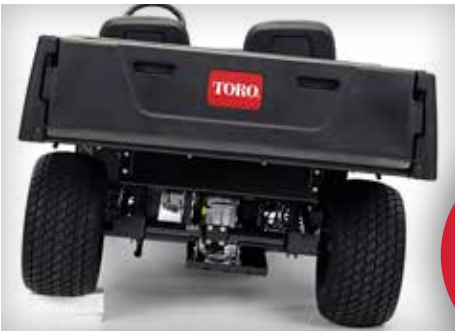
ACTIVE IN-FRAME TWISTER JOINT The Workman MDX innovative Active In-Frame Twister Joint allows each axle to react independently to the terrain.
