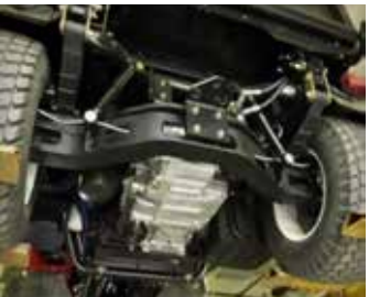
DEDION REAR AXLE The DeDion rear axle, standard on the Workman HDX-D , isolates the engine, transmission and main frame from all load forces, eliminating stress to these main components.
