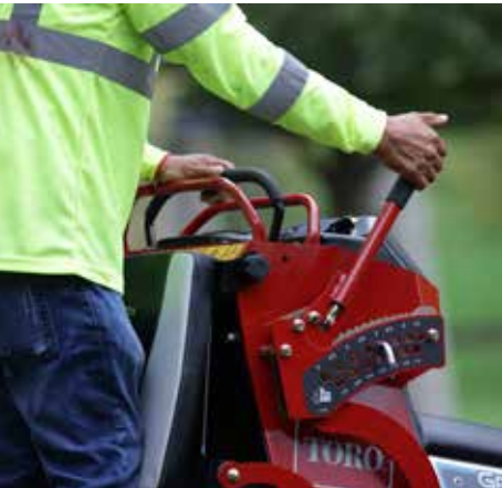
EASY ADJUSTMENT Adjust height-of-cut from the operator platform.
