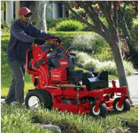
2-IN-1 VERSATILITY Toro's fold-up operator platform allows conversion of the GrandStand to a walk-behind. Just lower it back down to ride—no need to switch mowers.
