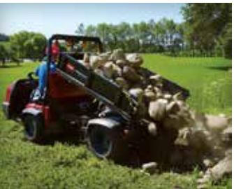
CARGO BED CAPACITY The Workman HDX-D cargo bed capability up to 1,293 kg (2,851 lbs). The Workman MDX cargo bed capability up to 567 kg (1,250 lbs).
