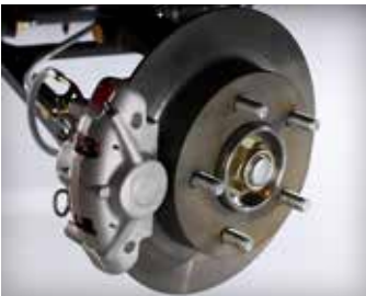
DISC BRAKES The Workman HD 4 wheel hydraulic disc brakes provide greater stopping power and easier servicing than traditional drum brakes.
