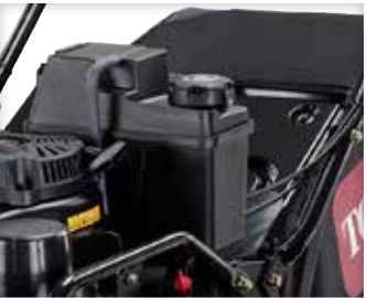
LONG RANGE FUEL TANK Saves time on re-fuelling with a 3.8 L fuel tank.
