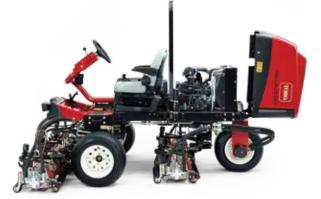
Simplified tractor design with a Tier 4 compliant engine, without the expense or complexity of larger engines that require Tier 4 after treatment systems, saves money in fleet maintenance expenses.
