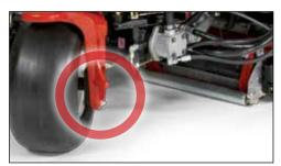
Jack points on all three wheels make removal of front and rear tires a breeze, and fluid sight levels on hydraulic and fuel tanks make daily visual maintenance checks fast and easy.
