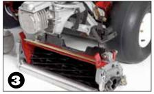
**Remove cutting units in minutes.** Facilitate routine maintenance activities like reel sharpening, simplify repairs and adjustments, and make it easy to change out seasonal accessories such as thatching reels or greens trirollers. Fast and easy cutting unit removal eliminates the need for a maintenance lift in your shop!
